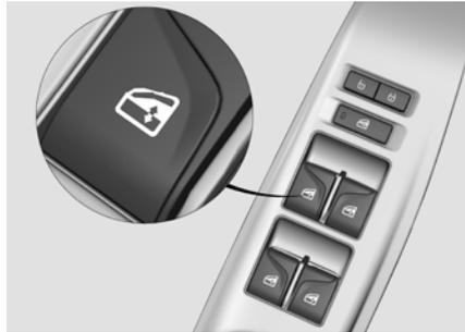
To open or close the window, press down or pull up the front end of corresponding switch to stop position.
